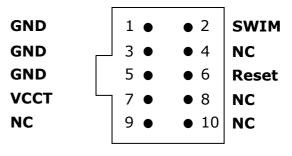
The signal outputs of the 10-pin interface are the same as for the 4-pin connector. Therefore, if needed for a specific hardware, an adapter cable can be soldered by using a 4-pin "Ernie" cable and soldering one end to a 10-pin header.
