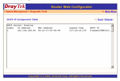
You can easily identify your Flasher by its host ID (in this case FLASHER351100023) and by its MAC addr which always starts with: 00-22-C7-03-XX-XX where XX depends on the last five digits of the serial number of your Flasher. In this case the serial number of the connected Flasher is 351100023 (0x0017), so its MAC address is: 00-22-C7-03-00-17.
