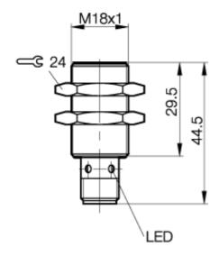
Inductive Sensors BES 516-326-E5-C-S 4 M18x1 x 44.5 normally-open Sn=5mm shielded
