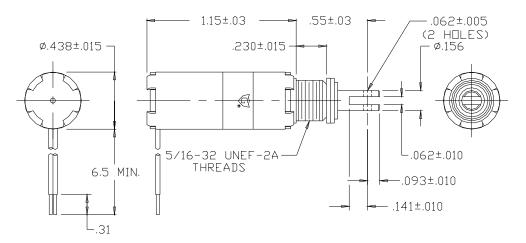
Solenoid shown energized and fully seated. Supplied with mounting bracket, hex nut and lockwasher (not shown).
