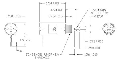
Solenoid shown energized and fully seated. Supplied with mounting bracket, hex nut and lockwasher (not shown). Spring kits are available (consult factory).
