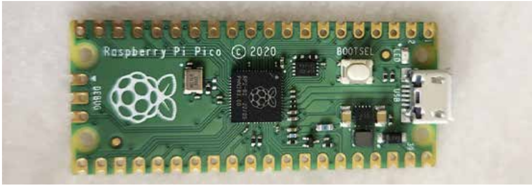
Figure 2. The Raspberry Pi Pico Board featuring the RP2040
