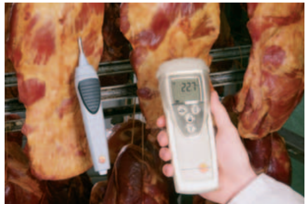
Measurement of penetration temperature using a wireless probe
