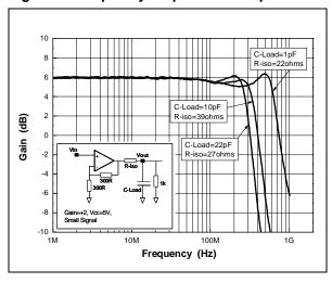
Figure 4: Frequency response, negative gain
