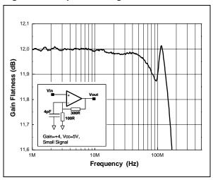
Figure 3: Frequency response vs. capa-load
