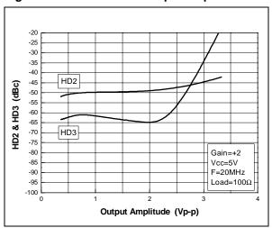
Figure 16: Distortion vs. output amplitude
