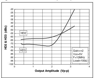
Figure 15: Distortion vs. output amplitude
