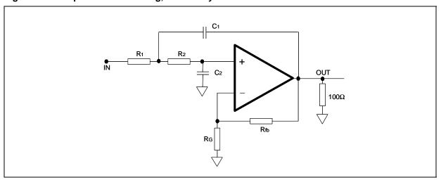
From the resistors  $R_{fb}$  and  $R_{G}$  we can directly calculate the gain of the filter in a classical non-inverting amplification configuration:
