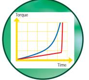
The red line indicates the steep increase in torque with hard applications, e.g. in metal.
