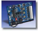
This board provides a cost-effective method of evaluating and developing sensored or sensorless BLDC motor control applications. A 28-pin, dsPIC30F3010 device is used with this board.
