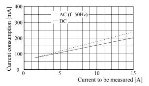
Figure 4. Typical probe consumption
