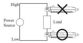
Figure 5. Low-voltage side of the circuit
