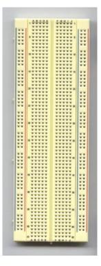
Material: high class POM plastic steel, Dimension: 166 x 54.5 x 11mm, Distribution strips: 2, Distribution holes: 200, Terminal strips: 1, Terminal holes: 630, Aluminum plate thick: 0.4, With paper box or skin packing
