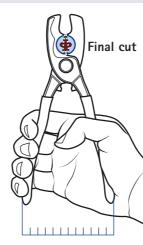
Final cut: if higher handforce is required, an additional cut can be done with the cutting edge profile near the joint. Initial cut with the upper cutting edge – final cut with the lower cutting edge
