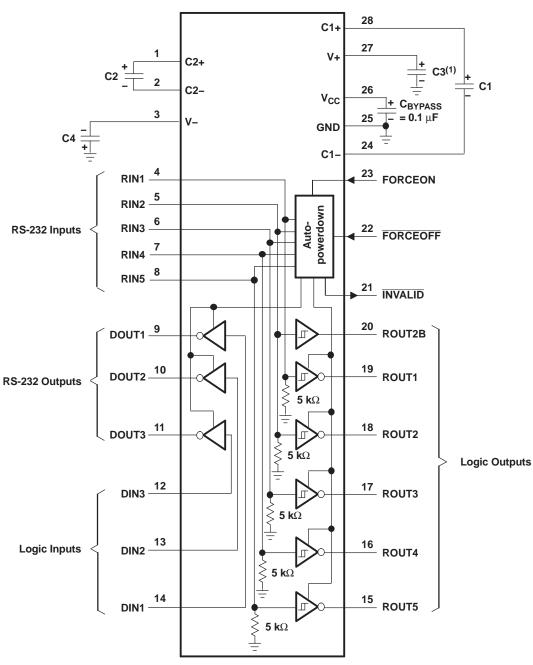
(1) C3 can be connected to  $V_{CC}$  or GND.
