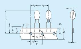
'B' wires for normal automatic insertion on 5mm pitch.
