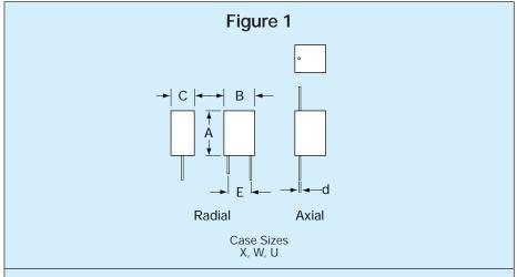
Leads – Leads are solder coated pure nickel wire suitable for soldering or welding. Tested in accordance with MIL-STD-202, Method 211, .010 diameter leads withstand a 1-lb. pull and .007 diameter leads an 8 oz. pull. All lead diameters withstand 5 rotations twist.
