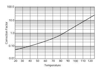
Figure 3. Correction factor to failure rate F for ambient temperature T for typical component (60% con. level).
