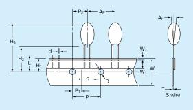
'S' and 'D' wire for special applications, automatic insertion on 2.5mm pitch.
