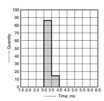
6. Distribution of release time Sample: CP1-12V, 100pcs Ambient temperature: 20°C 68°F \* Without diode
