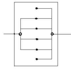
Terminals 1 and 6 are frequently unused, 2 pair (4 wire) cable is normally used in these installations. All wiring in parallel, i.e. terminal 1 on master socket to terminal on secondary socket, terminal 2 to terminal 2, etc.
