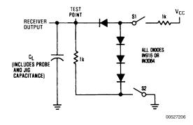
FIGURE 1. Receiver Propagation Delay Test Circuit
