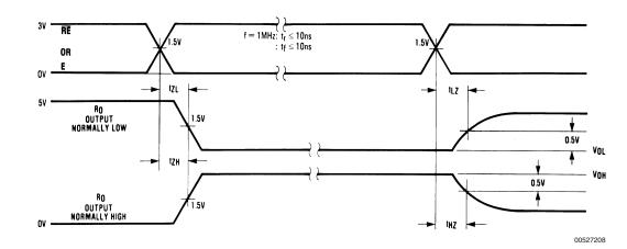
FIGURE 3. Receiver Enable/Disable Propagation Delay Timing
