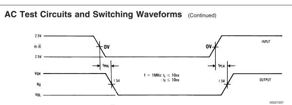
Differential input voltage may be realized by grounding  $\overline{\text{RI}}$  and pulsing RI between +2.5V and –2.5V
