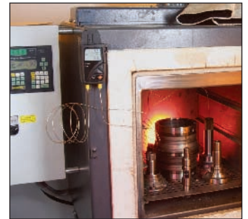
Fast measurement of high temperatures, e.g. in a hardening furnace
