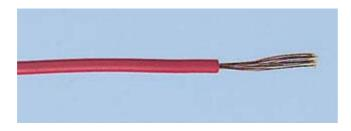
Flexible switchgear and control wire, manufactured in accordance with BS6231, UL1015 and CSA TEW 105°C. Applications include the wiring of switch and control panels and in motor starters and controllers..
