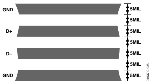
Figure 29. Arrangement of Signal Tracks
