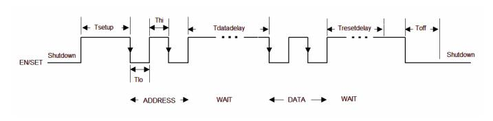
Figure 1. EN/SET One Wire Addressable Timing Diagram
