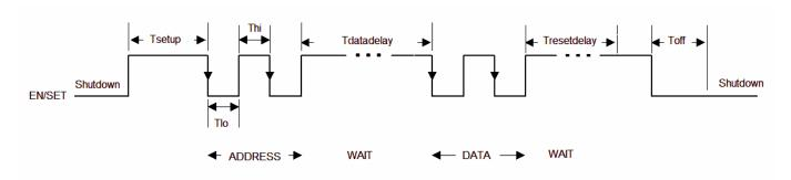
Figure 3. EN/SET One Wire Addressable Timing Diagram
