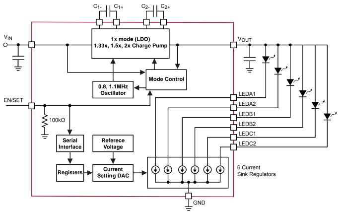
Figure 2. CAT3636 Functional Block Diagram
