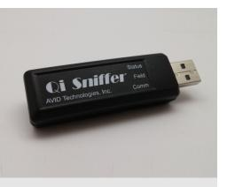
The Qi Sniffer is a USB device that can be placed near a Qi compliant wireless power system (TX and RX pair) and used to capture the wireless communication packets and other system operating information. The Qi Sniffer detects, demodulates, and decodes comm. data with different polarities and bit rates.
