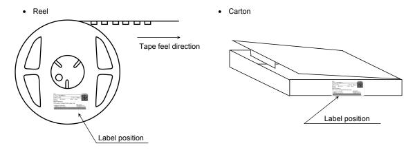
The aluminum package in which the reel is supplied also has the label attached to center of one side.
