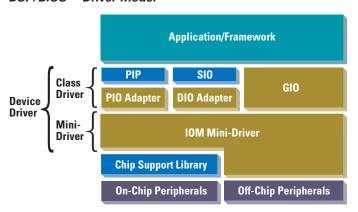
The DDK defines a two-level driver model and additional application-level APIs that simplify development of device drivers.
