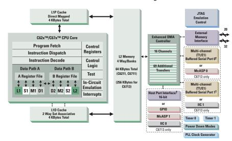
The C6211 and C6711 DSPs' innovative two-level cache memory structure enables a breakthrough in system cost/performance. \*The C6712 DSP features a 16-bit EMIF and no HPI. All C621x and C671x devices are pin compatible. The C6713 DSP is a superset of the C6711 DSP and will include I2S, I2C and S/PDIF transmit support as well as enhanced memory space.
