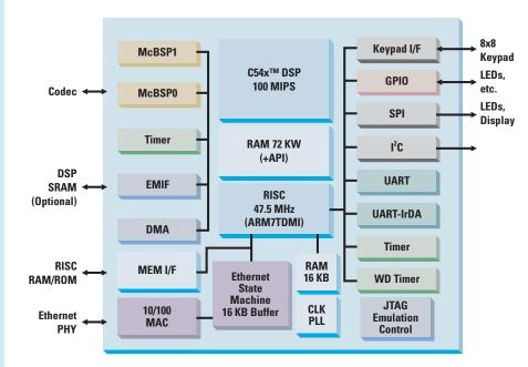
The system-level DSPs integrate C54x<sup>TM</sup> DSP with an ARM7 RISC and the most widelyused embedded operating systems. The C5470/C5471 DSPs deliver DSP-enabled performance for low-cost connected applications such as wireless data, smart pen pads, text-tospeech, voice recognition command control, access point controller, networked security, industrial control and emergency radio.
