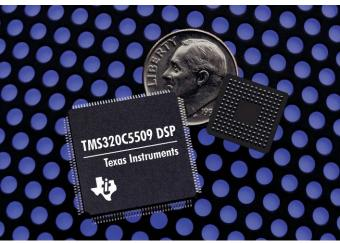
The ultra-small physical size (12 mm  $\times$  12 mm  $\times$  1.4 mm) of the C5000™ DSP MicroStar BGA (ball grid array) packaging can also help increase the performance per square inch for MIPS-intensive or spaceconstrained applications. The C5509 DSP is also pictured in a 144-pin LQFP.
