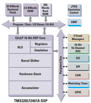
For high-performance industrial applications, the Flash-based LF2407A DSP includes peripherals such as a Controller Area Network (CAN) module to enable control of multiple motors by a single DSP.
