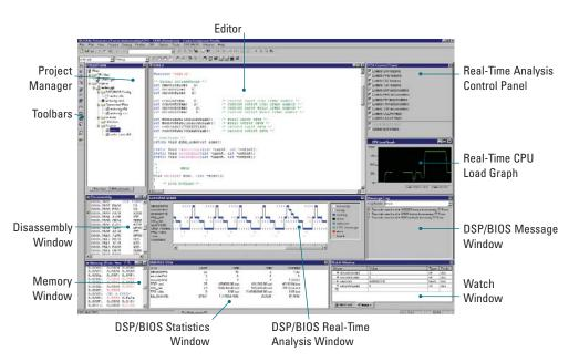
DSP/BIOS™ configuration and real-time analysis tools are included and are fully integrated with Code Composer Studio IDE.
