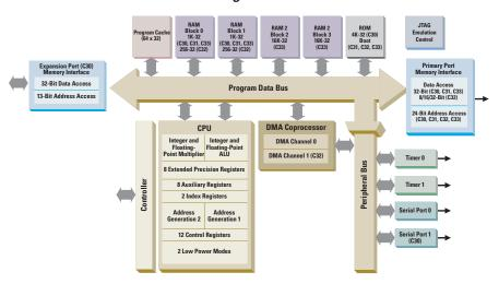
TMS320C3x DSPs offer extensive internal busing and up to 150-MFLOPS performance.
