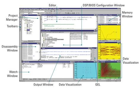
Code Composer Studio Development Tools feature all tools used in the development cycle working tightly together. Edit, build, debug and visualize.
