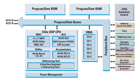
This block diagram of the TMS320C54x DSP is a comprehensive diagram showing all peripheral options. C54x™ DSPs are optimized to meet the performance, cost and low-power needs of wireless and wireline communications systems as well as emerging applications like IP phones, VoP and portable applications.
