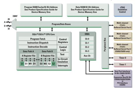
The fixed-point C6201 DSP is pin-for-pin compatible with the floating-point C6701 DSP offering easy code transfer resulting in significant savings in development, resource and manufacturing costs. Pin compatibility between the C6202, C6203 and C6204 DSPs allow for easy migration between several memory, price and performance options. The C6205 DSP is the first TI DSP with on-chip PCI.
