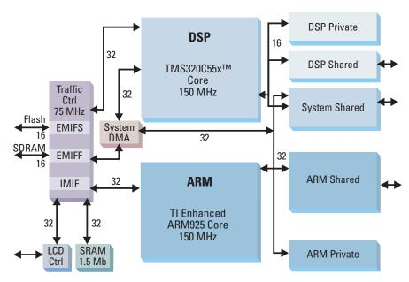
OMAP5910 processor diagram with ARM925 and C55x™ DSP cores and peripherals.
