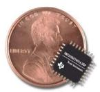
The TMS320LF2401A DSP packs a lot of power in an unbelievably small package. In only 49 mm², the TMS320LF2401A DSP provides 40 MIPS of processing power, a lightning-fast ADC with 500-ns conversion time, 8K of sectored Flash with code security, plus much more.
