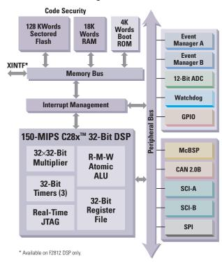
The F2810 and F2812 DSPs are the industry's first 32-bit control DSPs with on-board Flash memory and performance up to 150 MIPS.
