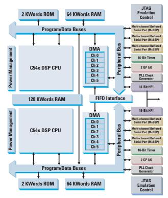
The C5420 and C5421 DSPs are dual-core DSPs targeted at carrier-class voice and video end equipments. The C5441 DSP features four C54x DSP cores on a single piece of silicon, offering 532 MIPS and is targeted at high-channel-density solutions.
