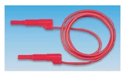
Silicone rubber test leads available in 1.0m or 1.5m lengths terminated at each end with 4mm shrouded stackable plugs. Spring loaded shroud retracts when inserted.
