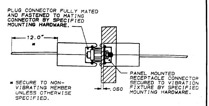
NOTE: RECEPTACLE CONNECTOR TO BE MOUNTED ON VIBRATION FIXTURE UNLESS OTHERWISE SPECIFIED.
