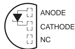
LP (TO-92/TO-226) PACKAGE (TOP VIEW)
