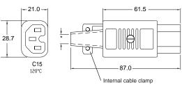
ø 7 mm for 1.0mm<sup>2</sup> cable ø 8.5 mm for 14 AWG cable 4784 Series, Angled 90°
