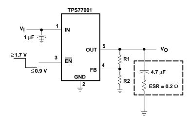
Figure 22. TPS77001 Adjustable LDO Regulator Programming
