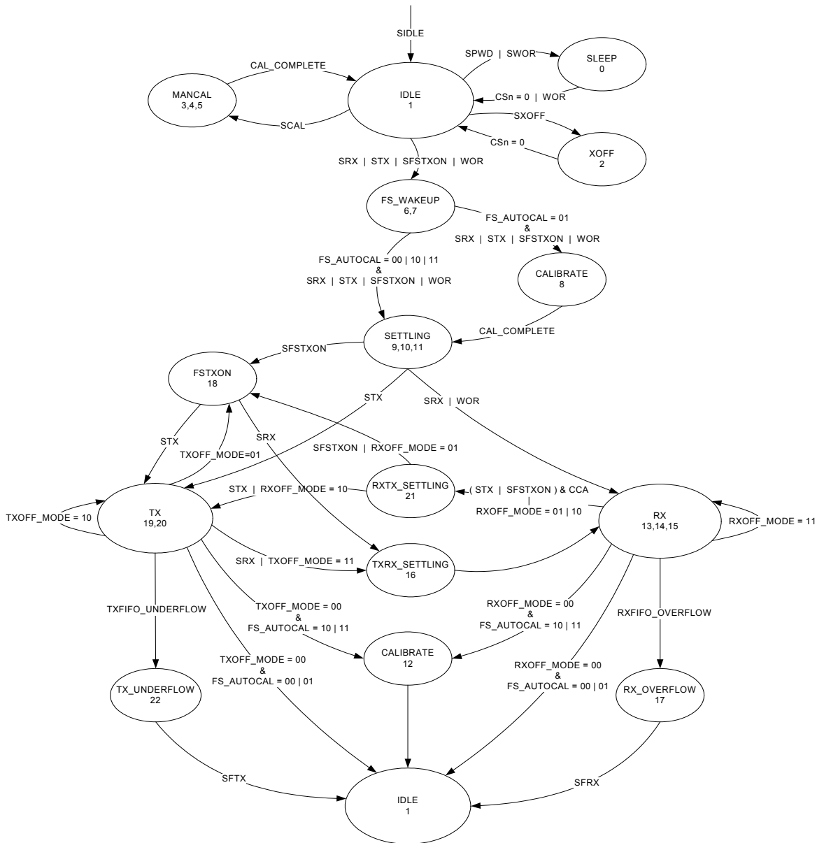
Figure 16: Complete Radio Control State Diagram
