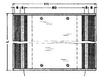
No solder point or component mounting is to be made in the area of the mechanical printed circuit board supports.
