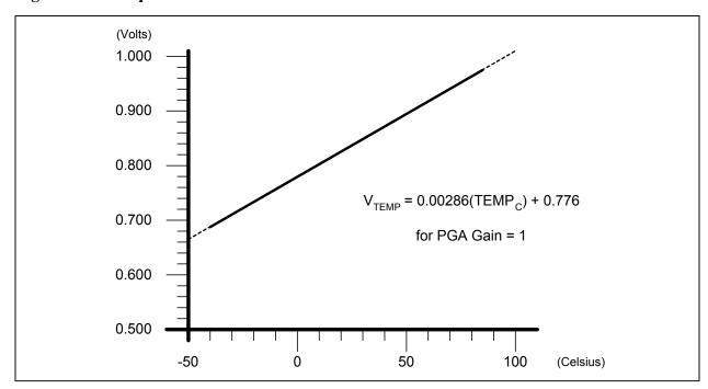
Figure 6.3. Temperature Sensor Transfer Function
