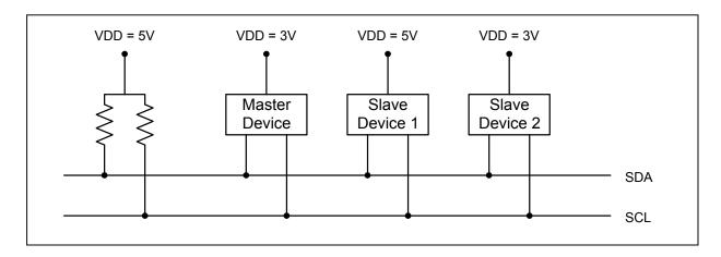
Figure 16.2. Typical SMBus Configuration
