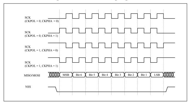
Figure 17.4. Data/Clock Timing Diagram
