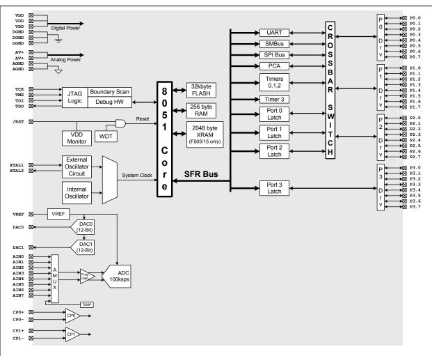
Figure 1.1. C8051F000/05/10/15 Block Diagram
