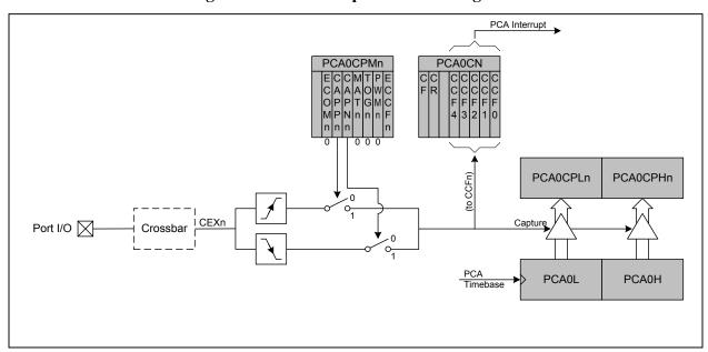
Figure 20.3. PCA Capture Mode Diagram
