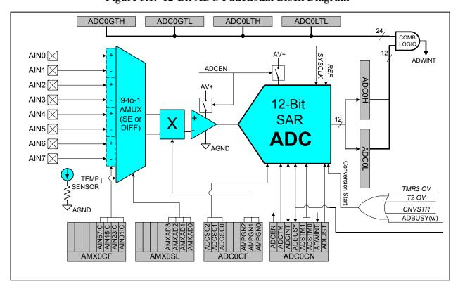
Figure 5.1. 12-Bit ADC Functional Block Diagram
