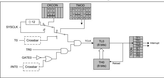
Figure 19.2. T0 Mode 2 Block Diagram
