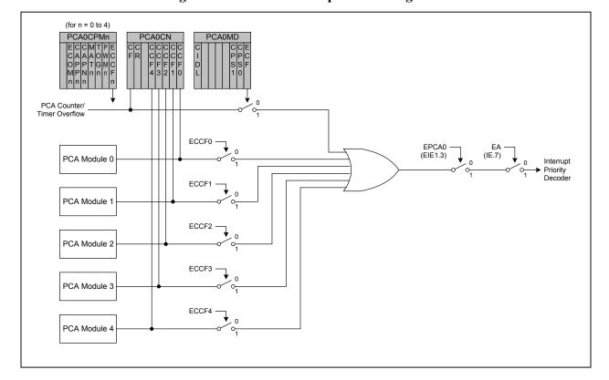
Figure 20.2. PCA Interrupt Block Diagram
