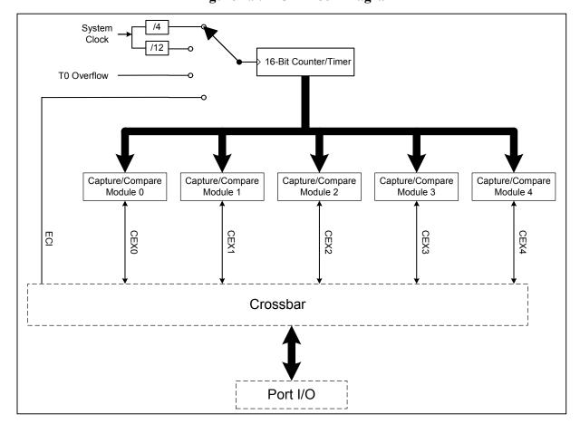
Figure 1.9. PCA Block Diagram
