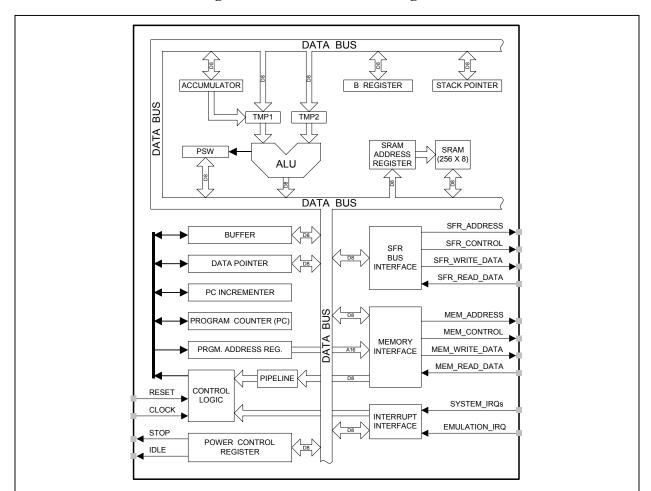
Figure 10.1. CIP-51 Block Diagram
