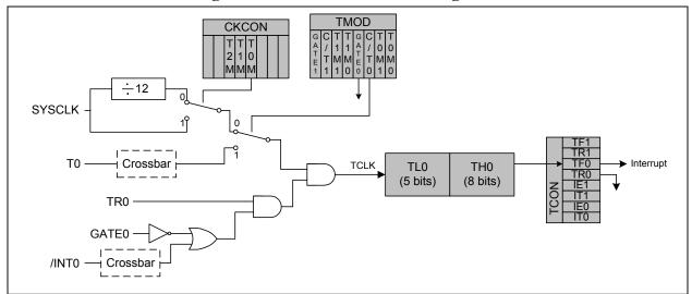
Figure 19.1. TO Mode 0 Block Diagram
