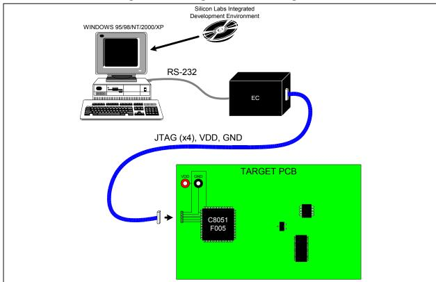
Figure 1.7. Debug Environment Diagram
