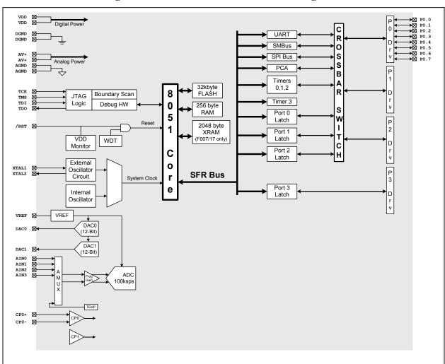
Figure 1.3. C8051F002/07/12/17 Block Diagram
