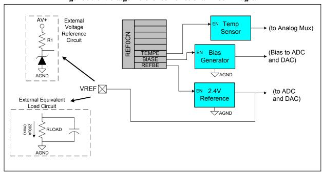
Figure 9.1. Voltage Reference Functional Block Diagram
