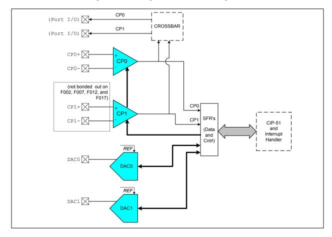
Figure 1.11. Comparator and DAC Diagram
