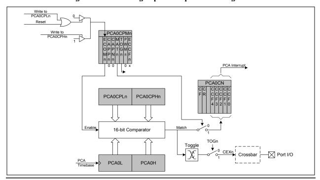
Figure 20.5. PCA High Speed Output Mode Diagram
