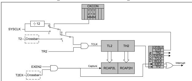
Figure 19.11. T2 Mode 0 Block Diagram
