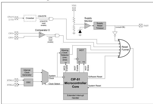
Figure 1.5. On-Board Clock and Reset
