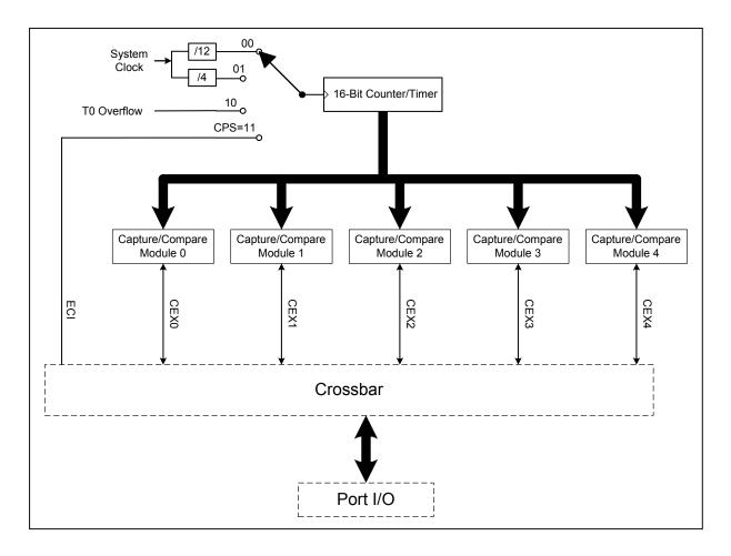
Figure 20.1. PCA Block Diagram
