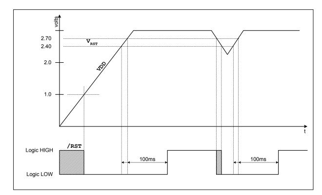
Figure 13.2. VDD Monitor Timing Diagram
