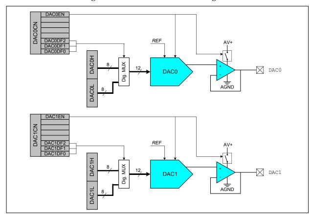
Figure 7.1. DAC Functional Block Diagram
