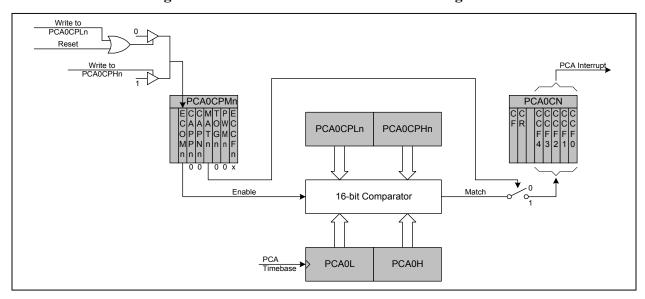
Figure 20.4. PCA Software Timer Mode Diagram
