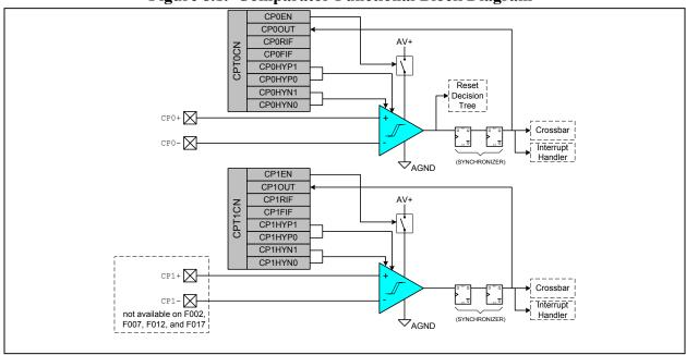
Figure 8.1. Comparator Functional Block Diagram
