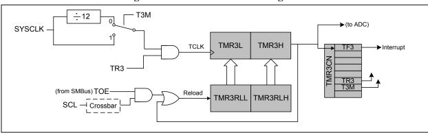
Figure 19.19. Timer 3 Block Diagram
