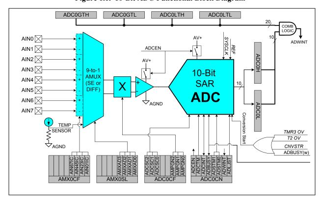
Figure 6.1. 10-Bit ADC Functional Block Diagram
