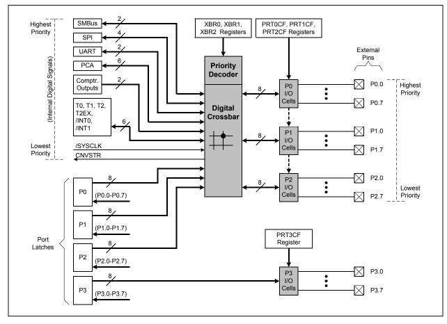
Figure 15.1. Port I/O Functional Block Diagram
