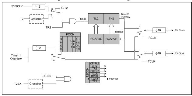
Figure 19.13. T2 Mode 2 Block Diagram
