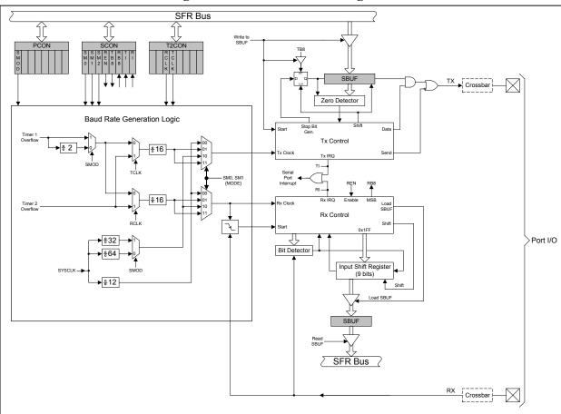
Figure 18.1. UART Block Diagram
