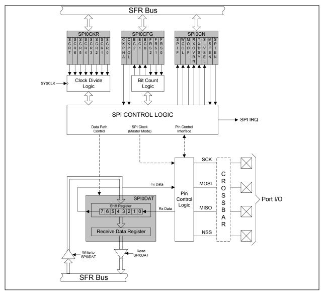
Figure 17.1. SPI Block Diagram
