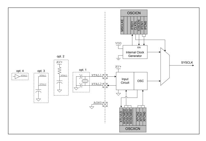
Figure 14.1. Oscillator Diagram
