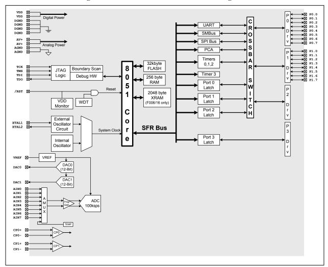
Figure 1.2. C8051F001/06/11/16 Block Diagram
