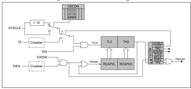
Figure 19.12. T2 Mode 1 Block Diagram
