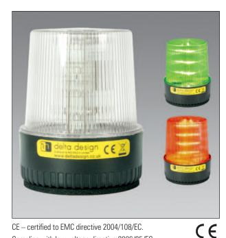
CE – certified to EMC directive 2004/108/EC. Complies with low voltage directive 2006/95/EC. High voltage transient and polarity reversal protected. Operating temperature:  $-20^{\circ}$ C to  $+55^{\circ}$ C.
