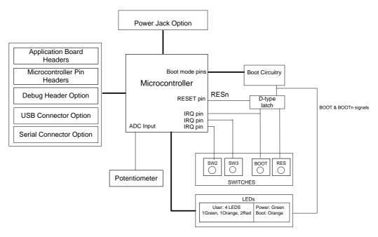
Figure 5.1: Block Diagram
