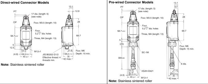
Roller Lever Plungers WL are Standard Models and WL01 are Microload Models.
