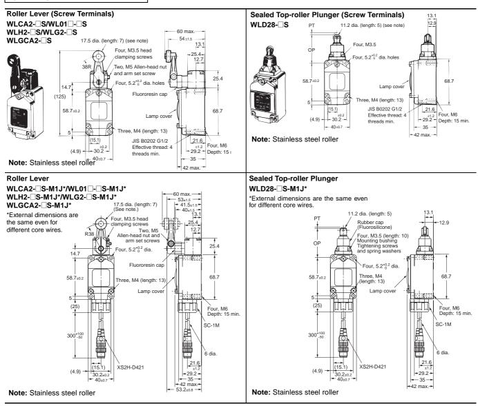
Note: Unless otherwise indicated, a tolerance of  $\pm 0.4$  mm applies to all dimensions.
