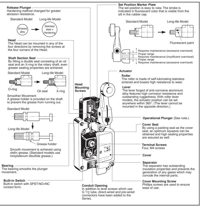
Note: By changing the direction of the operational plunger, any one of the three operational directions (both sides, left, or right) can be selected. (Applicable only to the WLMGCA2-...)
