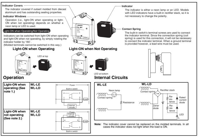
Note 1. Light-ON when operating means that the lamp lights when the Limit Switch contacts (NC) release, or when the actuator rotates or is pushed down. Light-ON when not operating means the lamp remains lit when the actuator is free, or when the Limit Switch contacts (NO) close when the actuator rotates 2. or is pushed down.
