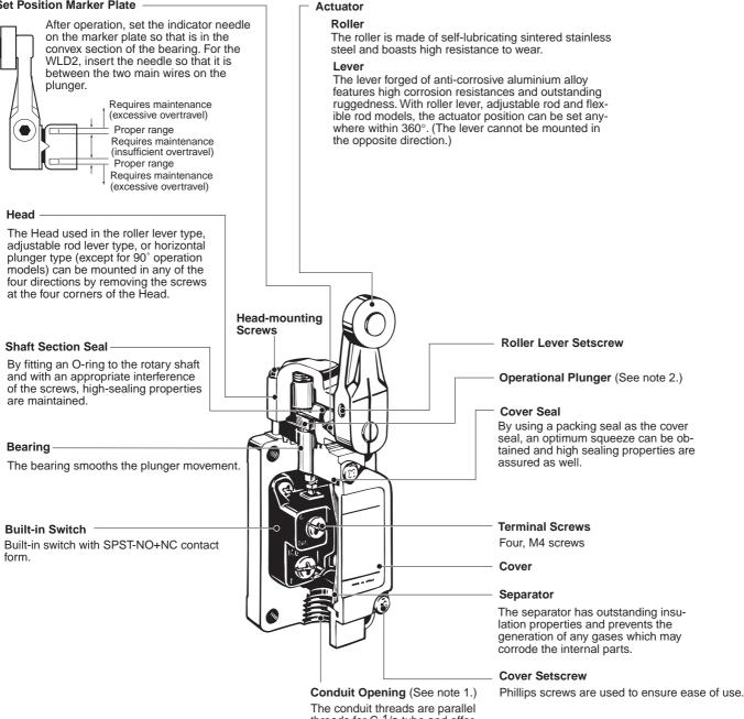
threads for G 1/2 tube and offer further increased sealing properties when used in conjunction with the SC connector.
