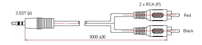
Jacket : 2/¢2.6 PVC Black Spiral : 2 x 28/0.1 Cu Insulation : 2/¢1.0 PE Red/White Inner Conductor : 2 x 9/0.12 Cu
