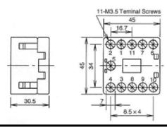
Plug-in Three-Phase Monitor Relays require a 600V-rated socket when used on system voltages greater than 300V.
