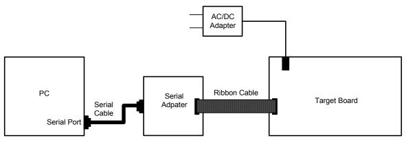
Figure 1. Hardware Setup
