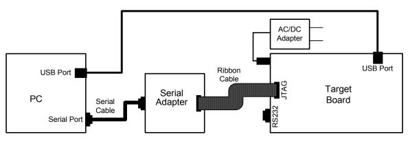
Figure 2. USB Application Hardware Setup
