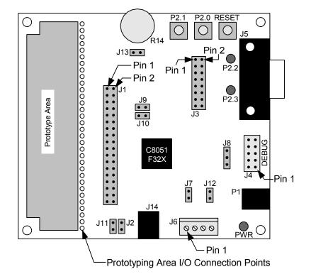
Figure 3. C8051F320 Target Board
