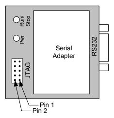
Figure 4. Serial Adapter DEBUG/JTAG Connector
