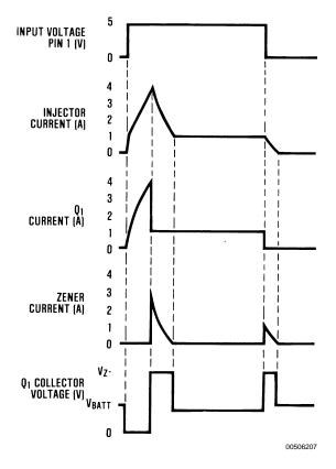
FIGURE 4. Circuit Waveforms
