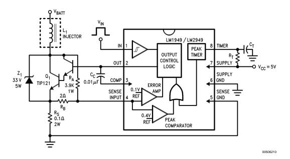
FIGURE 7. Switching Application Circuit
