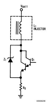
FIGURE 5. Alternate Configuration for Zener Z<sub>1</sub>
