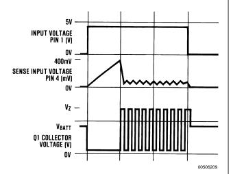
FIGURE 6. Switching Waveforms
