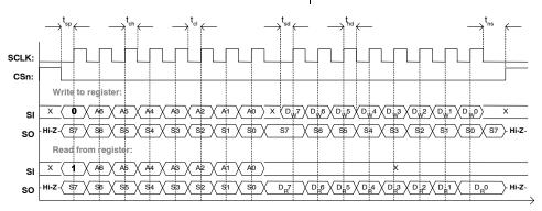
Figure 6: Configuration registers write and read operations
