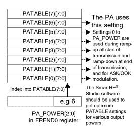
Figure 14: PA\_POWER and PATABLE
