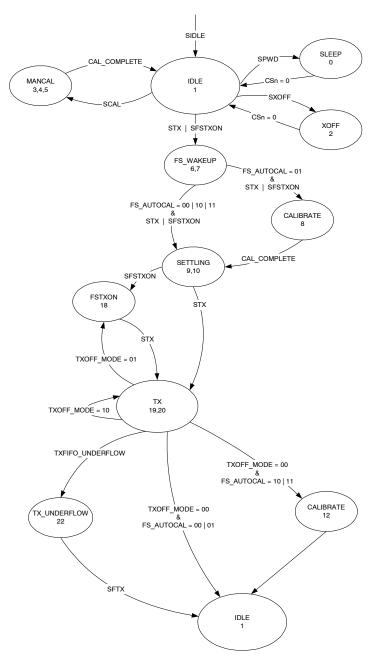
Figure 10: Complete Radio Control State Diagram
