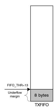
Figure 13: Example of FIFO at threshold
