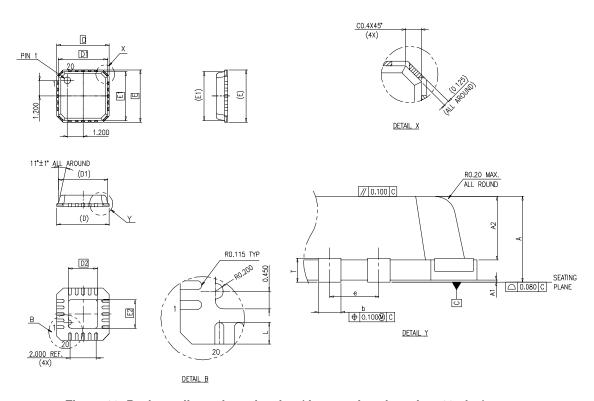
Figure 16: Package dimensions drawing (the actual package has 16 pins)
