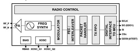
Figure 2: **CC1150** Simplified Block Diagram
