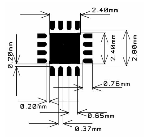
Figure 17: Recommended PCB layout for QLP 16 package
