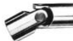
Single joint fitted with needle roller bearings. The journals are machined integral with the central block.
