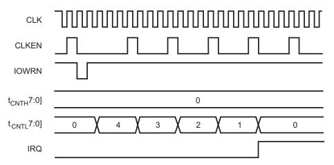
Figure 19. PRT Single Pass Mode Operation Example
