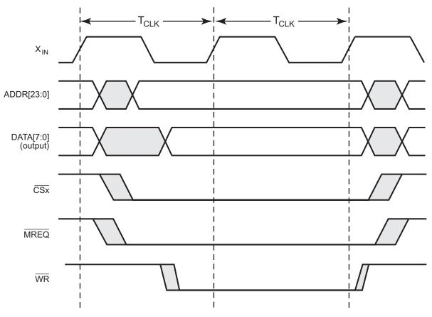
Figure 54. Wait State Timing for Write Operations
