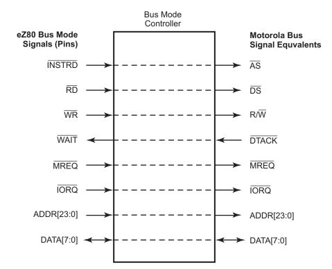
Figure 14. Motorola Bus Mode Signal and Pin Mapping
