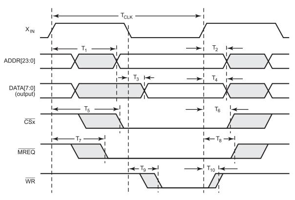
Figure 50. External Memory Write Timing
