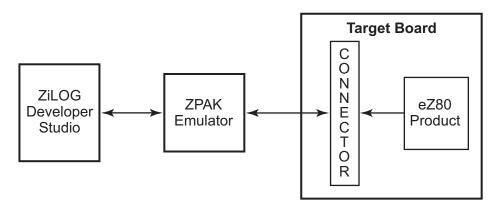
Figure 35. Typical ZDI Debug Setup
