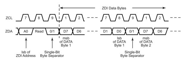
Figure 43. ZDI Block Data Read Timing
