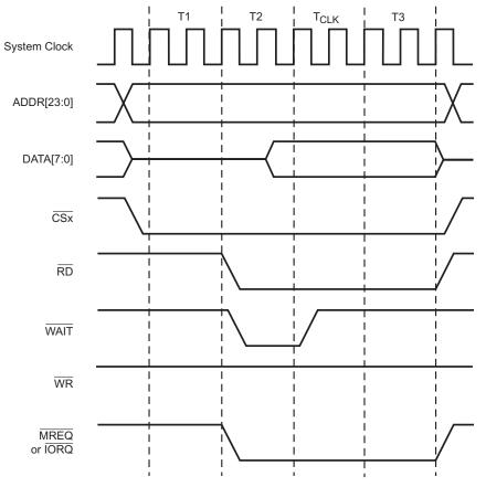
Figure 7. Z80 Bus Mode Read Timing Example
