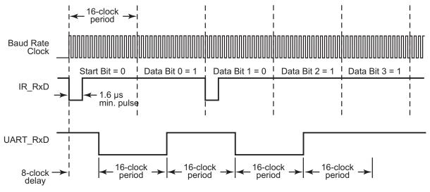
Figure 26. Infrared Data Reception
