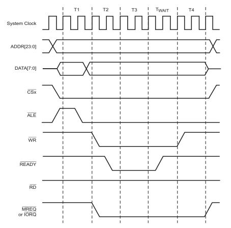
Figure 13. Intel<sup>™</sup> Bus Mode Write Timing Example (Multiplexed Address and Data Bus)
