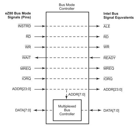
Figure 9. Intel<sup>™</sup> Bus Mode Signal and Pin Mapping
