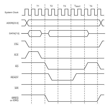
Figure 12. Intel<sup>™</sup> Bus Mode Read Timing Example (Multiplexed Address and Data Bus)
