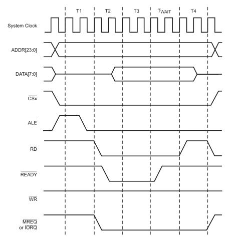
Figure 10. Intel<sup>™</sup> Bus Mode Read Timing Example (Separate Address and Data Buses)
