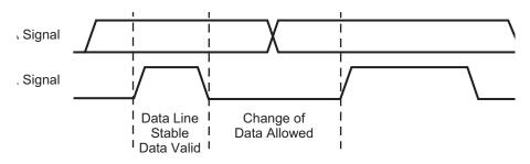
Figure 30. I<sup>2</sup>C Clock and Data Relationship
