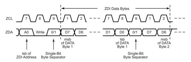
Figure 41. ZDI Block Data Write Timing
