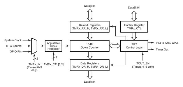
Figure 18. Programmable Reload Timer Block Diagram
