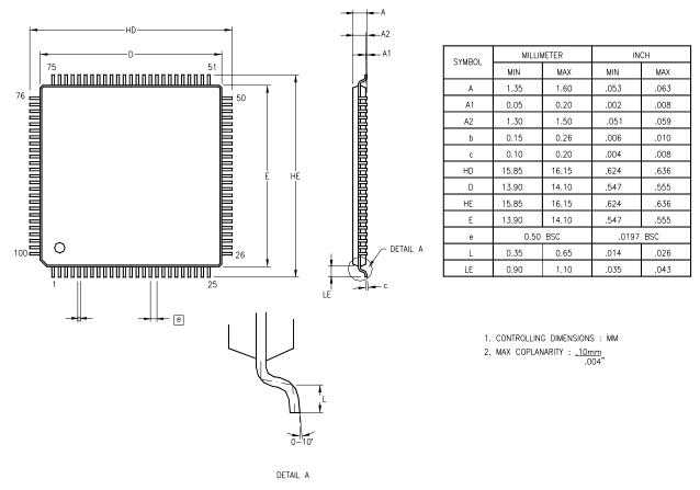
Figure 57. 100-Lead Plastic Low-Profile Quad Flat Package (LQFP)
