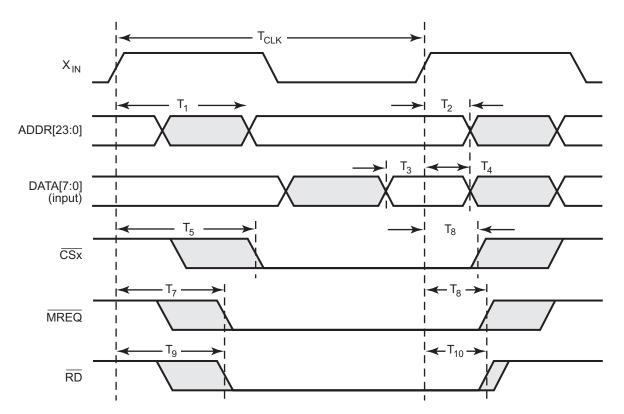
Figure 49. External Memory Read Timing
