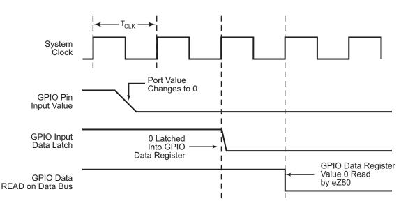
Figure 55. Port Input Sample Timing
