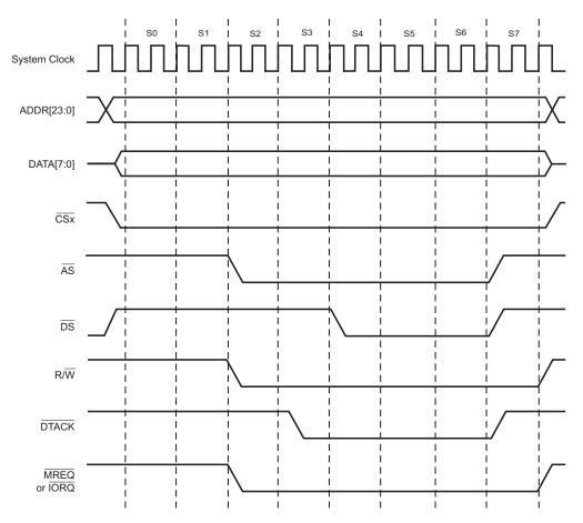
Figure 16. Motorola Bus Mode Write Timing Example
