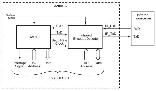
Figure 24. Infrared System Block Diagram
