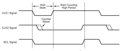
Figure 34. Clock Synchronization In I<sup>2</sup>C Protocol
