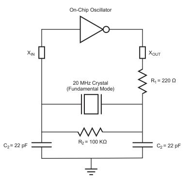
Figure 44.Recommended Crystal Oscillator Configuration (20MHz operation)
