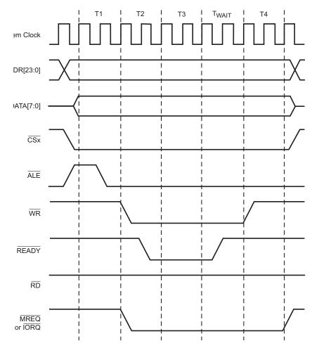
Figure 11. Intel<sup>™</sup> Bus Mode Write Timing Example (Separate Address and Data Buses)
