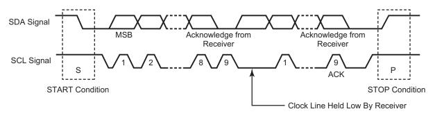
Figure 32. I<sup>2</sup>C Frame Structure
