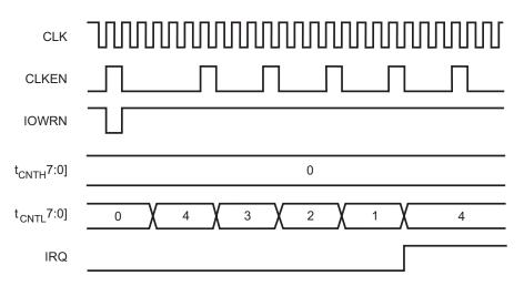
Figure 20. PRT CONTINUOUS Mode Operation Example
