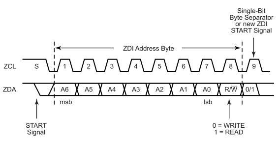
Figure 39. ZDI Address Write Timing
