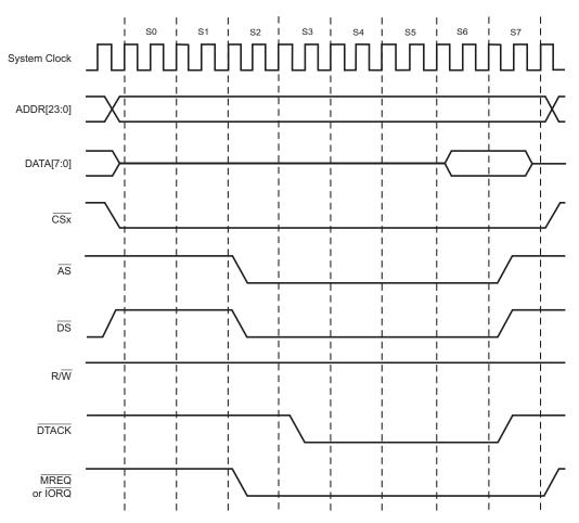
Figure 15. Motorola Bus Mode Read Timing Example
