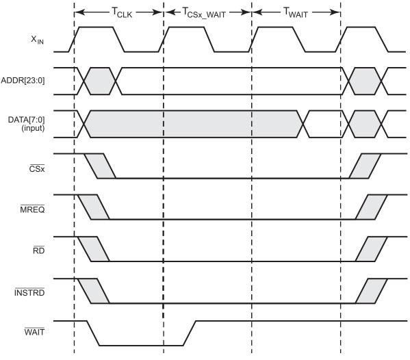
Figure 6. Wait State Operation Example (Read Operation)
