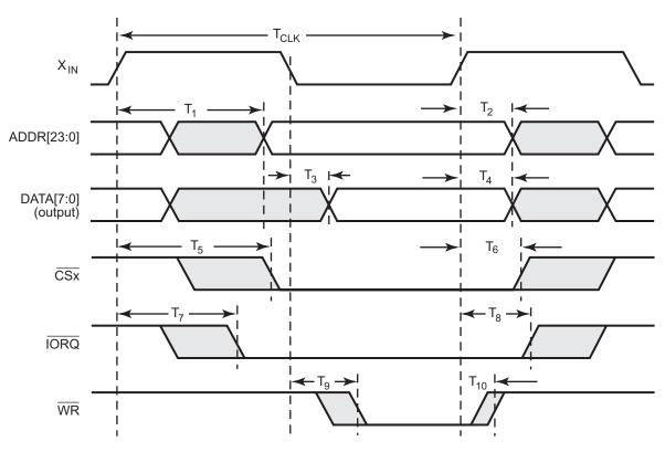
Figure 52. External I/O Write Timing
