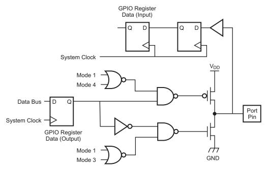
Figure 3. GPIO Port Pin Block Diagram
