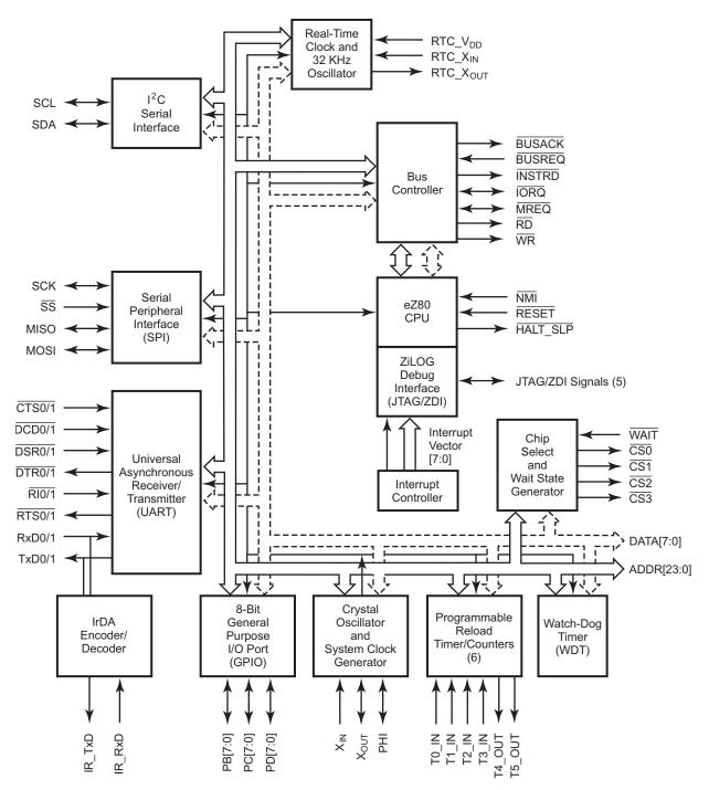
Figure 1. eZ80L92 Block Diagram
