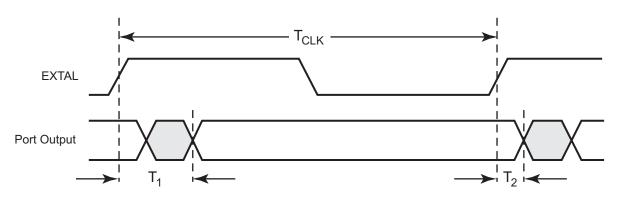
Figure 56. GPIO Port Output Timing
