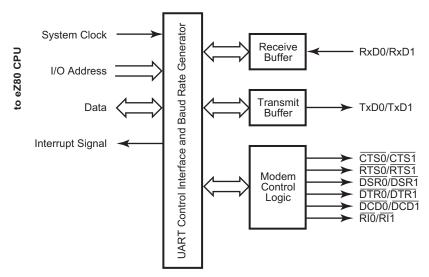
Figure 23.UART Block Diagram
