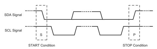
Figure 31. START and STOP Conditions In I<sup>2</sup>C Protocol
