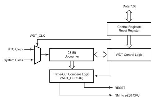
Figure 17. Watch-Dog Timer Block Diagram
