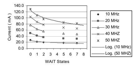
Figure 48.I<sub>CC</sub> vs. WAIT (Typical @ 3.3V, 25°C)
