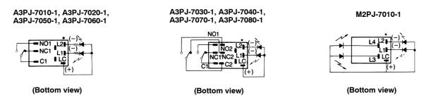
$\ast$  With the single screen type, connect an LED across terminals LC and L2.
