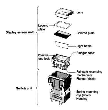
\* With the LED type, an LED is incorporated in the plunger case. With the lamp type, the lamp holder and plunger case are independent units. Insert a T-3/4 lamp in this holder.
