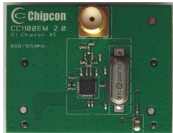
Figure 6: CC1100EM reference design, 868/915 MHz
