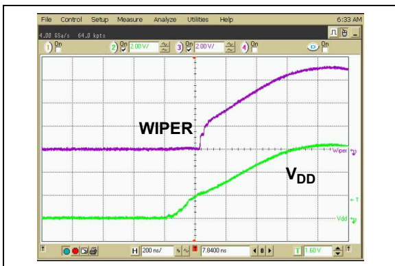
FIGURE 2-45: 50 k \Omega – Power-Up Wiper Response Time.
