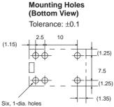
ALL DIMENSIONS SHOWN ARE IN MILLIMETERS. To convert millimeters into inches, multiply by 0.03937. To convert grams into ounces, multiply by 0.03527.
