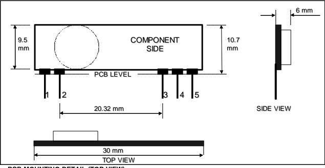
PCB MOUNTING DETAIL (TOP VIEW)
