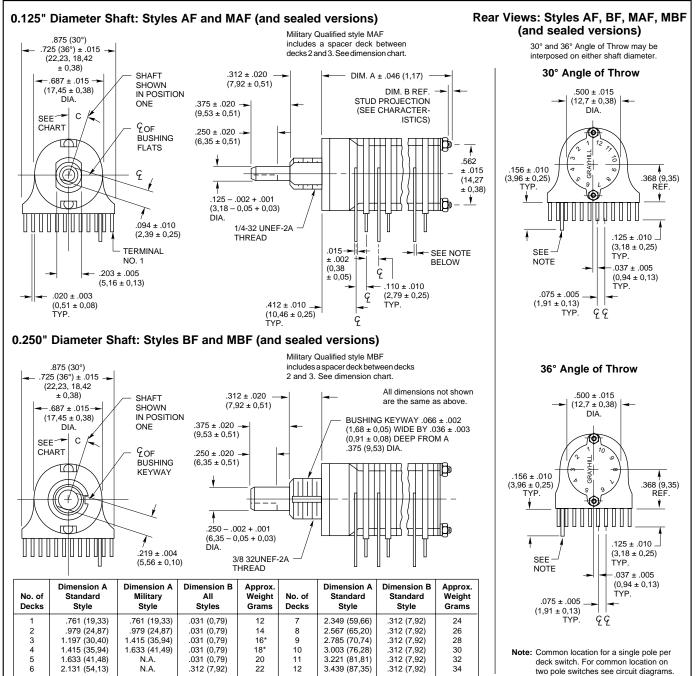
$\begin{array}{l} \textbf{Angle C} \text{ is } 15^{\circ} \text{ in } 12 \text{ position switches and } 18^{\circ} \text{ in } 10 \text{ position switches.} \\ ^{\star} \textbf{Military style switch is } 18 \text{ grams for } 3 \text{ decks and } 20 \text{ grams for } 4 \text{ decks.} \end{array}$
