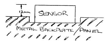
\*N.B. Both of these sensors can be surface mounted should you wish to do so. Also note that these diagrams are not to scale.
