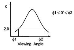
Contrast ratio K vs viewing angle \$\phi\$
