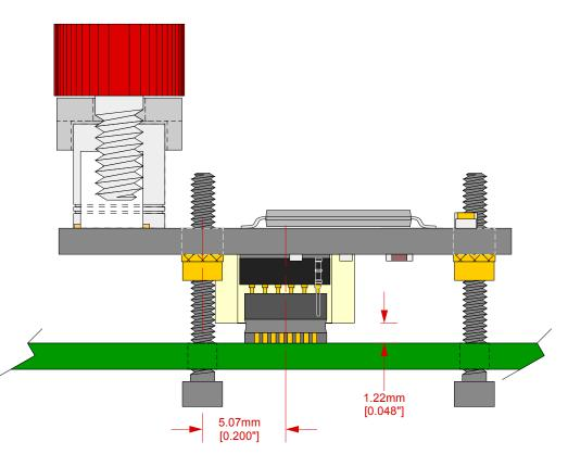
Side view: CY3250 - 24x23AQFN Pod on QFN32 foot
